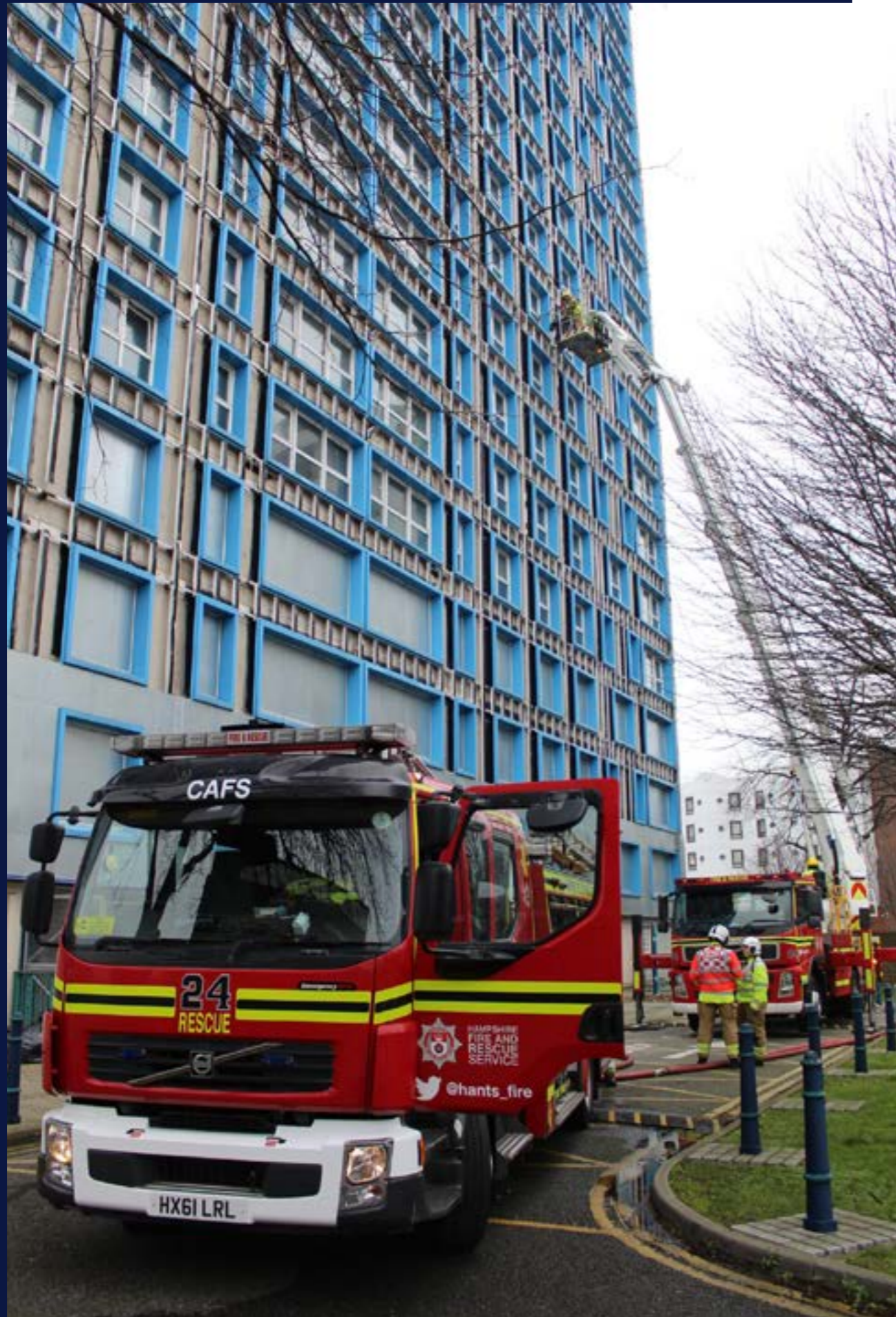
An aerial ladder platform operating outside a high-rise building in Portsmouth
